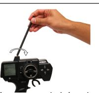
Install antenna into the hole in the top of the transmitter. Pull antenna to its full extent. Thread antenna into the transmitter.
