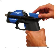
Remove battery cover by pulling gently away from starting pistol.
