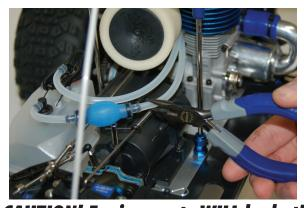
**CAUTION! Engine parts WILL be hot!**To shut your MGT 8.0 off, either squeeze fuel line with fingers or use pliers to cut the fuel flow to the carburetor. Once engine is off, turn off your vehicle, then turn off your transmitter.
