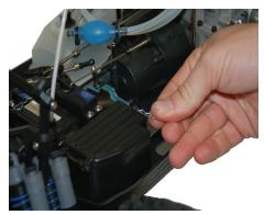
Use supplied clips to attach cover onto radio box.
