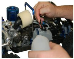
Lift the fuel tank lid and, using the supplied fuel bottle, fill the tank with fuel (not included).
