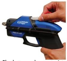
Plug battery pack connector into connector on top of starter.
