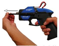
Remove starting bit from the holder on the side of the starting pistol.
