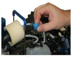
Prime the fuel by squeezing the blue bulb attatched to the fuel line.
