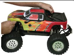
Attach body to chassis with the supplied body clips.
