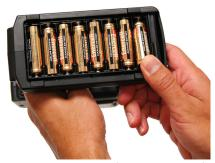
Insert 8 AA batteries (not included) into transmitter.
