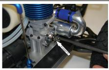
Slide the starter shaft through the side of your MGT 8.0 and into the hex starter on the back of the engine (body removed for clarification). Pull the trigger on the ProStart Starting Pistol to start engine.
