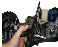
Move the switch on the transmitter to the ON position (blue LED will illuminate).
