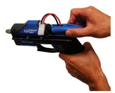
Slide wires through slot and close battery cover.
