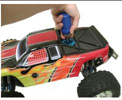
Insert the glow igniter into the head of the engine. Make sure it 'grabs' the glow plug.
