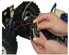
Insert 4 AA batteries or charged 5-cell NiMh pack into harness and install into radio box (not included).
