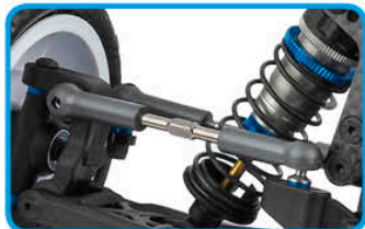
Updated ball cups and turnbuckles for precise adjustments and durability
