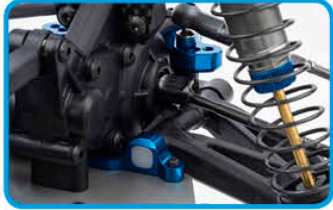
Lightweight and durable aluminum C plate and aluminum ball stud mount
