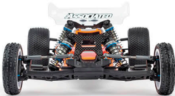
Gull wing arms, wide front tower Lower CG and increased on-power steering
