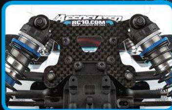
Graphite shock towers with multiple shock mounting positions
