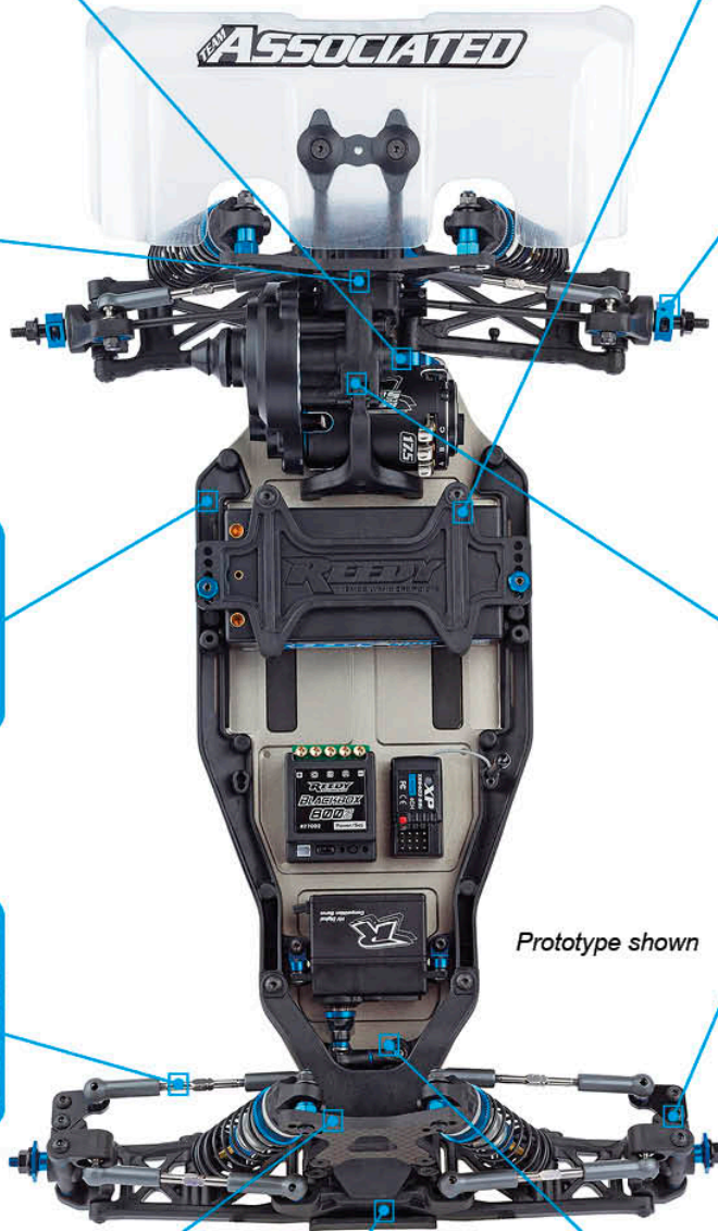
Adjustable battery hold-down strap allows weight bias tuning
