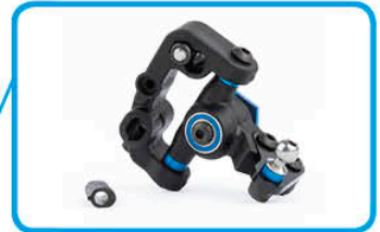
One-piece steering blocks with bolt-on Ackermann plate
