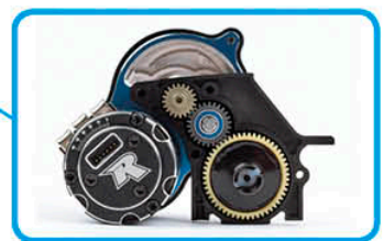
3-gear Stealth™ transmission with lightweight aluminum top shaft
