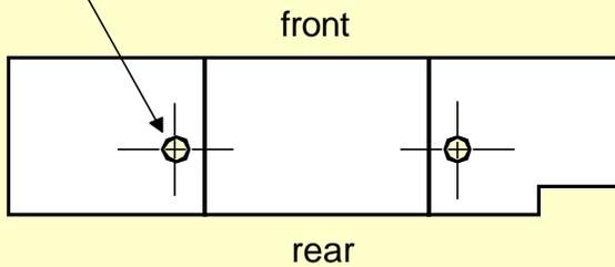
6. Install onto rack, washers underneath cover.
