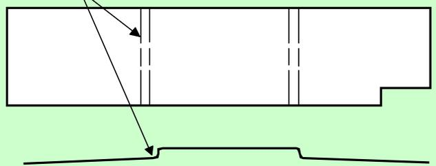
5. Drill 1/8" holes here and remove burrs.
