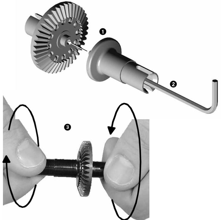
Rotate the hubs in opposite directions several times in between screwing in the diff bolt.
