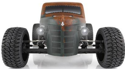
Factory-finished body with integrated LED lights, 2 front, 2 rear
