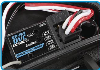
New DVC (Dynamic Vehicle Control) receiver featuring built-in adjustable gyro
